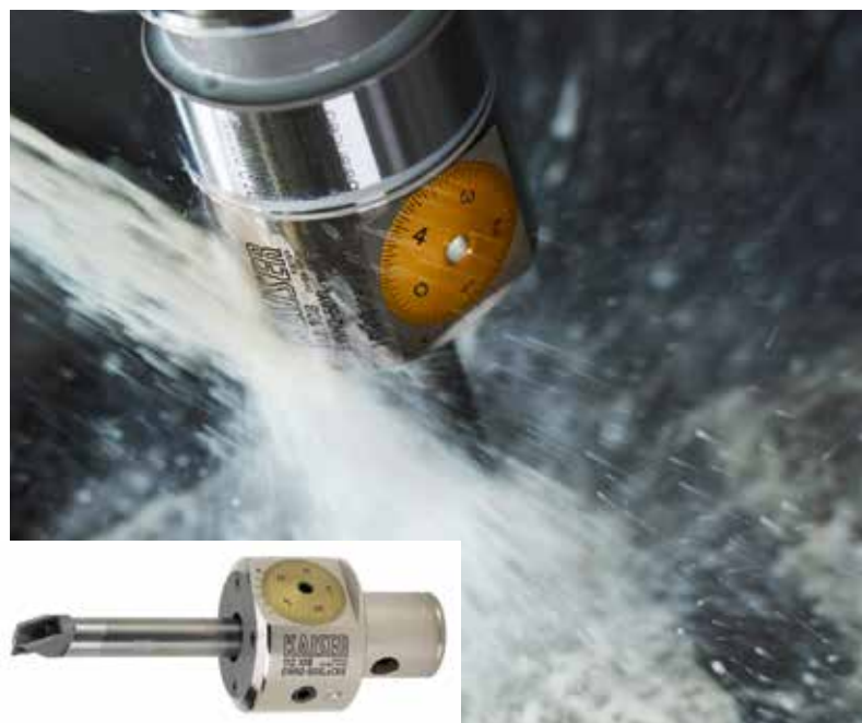
The test tool precision boring head EWN 2-50XL
