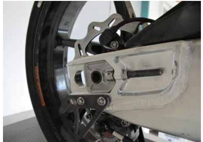
Rear axle of the Moto3 motorcycle; titanium screws and turnbuckles
