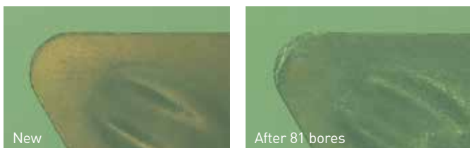
Competitor insert, TCMT110204, TiAlN (red curve)
