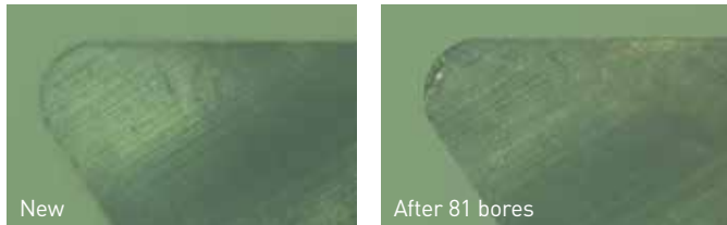
Insert KAISER, TCGT110204, AlCrN, art. no. 655.389 (blue curve)
