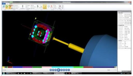
Simulation Builds Confidence: Nexxt Spine LLC, (Noblesville, Indiana) routinely compares STL data taken from Mastercam's model of the final machined part directly with the SolidWorks model. It is very much like inspecting the finished part before it has been manufactured.
