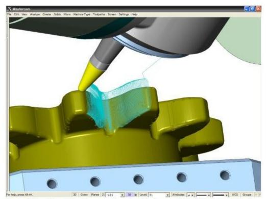
Five-Axis Gear Simulation: Heavy equipment part designs are typically delivered to Snyder Industries (Tonawanda, New York) as prints. One of the first things the company does is model everything in Mastercam—not just the part, but also the pallet setup and the machine itself. Being able to view a complete simulation of the part being manufactured gives the programmers confidence that the part can be manufactured at high speeds without encountering any interference.
