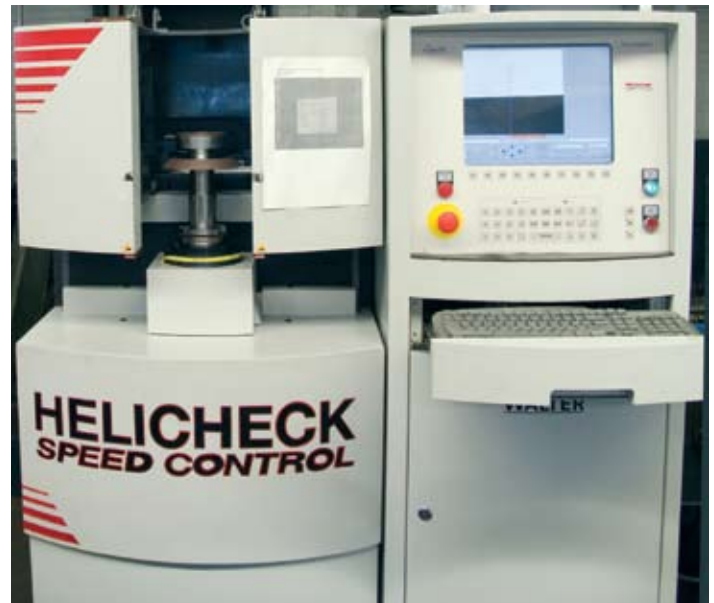
By measuring their grinding wheels in a Walter Helicheck, operators can get an extremely accurate simulation of the grind in advance, minimizing the need for tweaking on the machine
