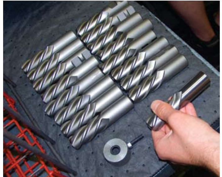
On the bench: Endmill blanks after they’ve been fully hardened and the shanks have been “drawn back” with an induction coil. In hand: After the shank has been ground to within a few tenths on a Studer. It’s more challenging than it appears because each shank has flats and varies in hardness from 50 to 67 Rockwell.
