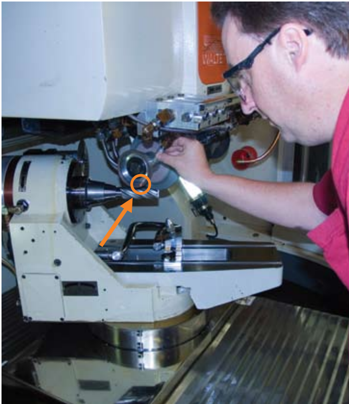
Operator Tim Wixted aims a coolant nozzle with a laser. The pipe is rigid in order to handle 200+ PSI. Tim reports that "Once you set the nozzle you're set until you change the wheels. They don't move."
