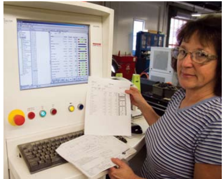
Operator Linda Wendt puts an endmill into a Walter Helicheck... Selects the parameters she wants to measure... Stands by as the machine does its magic... And reviews the certified inspection report. Graphics make it easy to see where each measured value falls within its tolerance band
