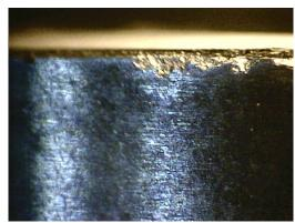
Chatter can be seen on the part finish. Frequently, you will be able to hear a chattering noise when the part is being machined. While this can be caused from many conditions, it is most frequently caused by the tool being above centerline.
