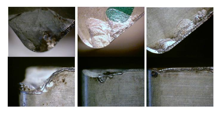
These inserts shows breakage across the top of the inserts from the cutting point.
