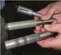
For General Tool ( TOP ), having an inventory of diamond tooling on hand allows the shop to respond quickly to composite-machining challenges. Both diamond-plated tools and carbide burrs are among the composites machining tools seen here at Reno Machine ( RIGHT ).
