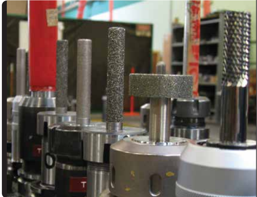
For General Tool ( TOP ), having an inventory of diamond tooling on hand allows the shop to respond quickly to composite-machining challenges. Both diamond-plated tools and carbide burrs are among the composites machining tools seen here at Reno Machine ( RIGHT ).
