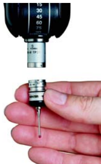
Stylus specification and configuration can affect the precision of measurement results
