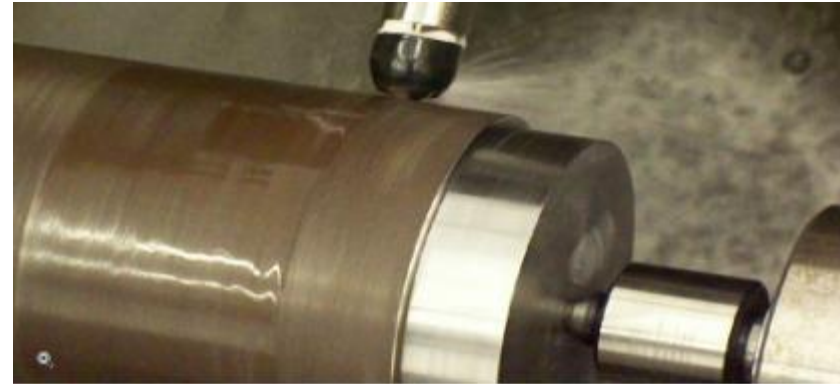
LPB Processing of a P110 coupling
